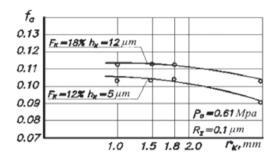
Fig. 7. Dependence of the adhesion component of the friction factor  $f_a$  on the bottom radius of a micro groove  $r_{\kappa}$
