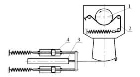
Fig. 2. Diagram of a tribometer (1 – sample; 2 – steel tape as a mating sample; 3 – friction torque transmitter; 4 – air dampers)
