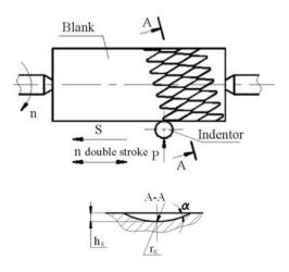
Fig. 1. A model of a partially regular microrelief formation by surface plastic deformation
