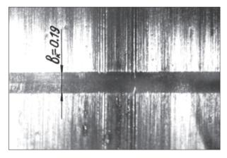
Fig. 14. Traces of penetration of micro asperity projections into the edges of micro grooves, which formed as a result of a micro seizure ( $h_k = 3 \mu m$ ,  $r_k = 1.5 mm$ )
