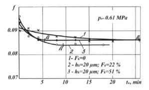
Fig. 12. Determining the time of the micro running-in completion  $t_w$  according to the stabilized friction factor f (point A)
