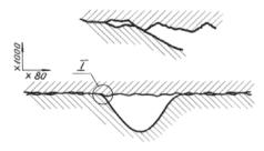
Fig. 10. The engagement of micro asperity projections with the edge of a micro groove in sliding friction
