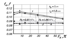
Fig. 5. Dependence of the adhesion component of the friction factor  $f_a$  (curves 1, 2) and the friction factor f after the micro running-in (curves 3, 4) on the relative area of micro grooves  $F_{\rm K}$
