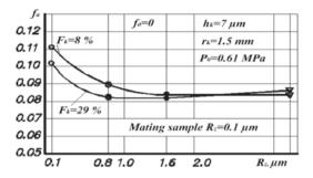
Fig. 8. Dependence of the adhesion component of the friction factor  $f_a$  on the relative area of micro grooves  $F_K$  at different sample roughness  $R_Z$
