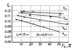
Fig. 6. Dependence of the adhesion component of the friction factor  $f_a$  on the relative area of micro grooves  $F_{\kappa}$  at a depth of micro grooves  $h_{\kappa}$ :  $h_{K1} = 20 \ \mu m$ ;  $h_{K2} = 11 \ \mu m$ ;  $h_{K3} = 7 \ \mu m$ ;  $h_{K4} = 3 \ \mu m$
