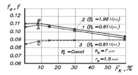
Fig. 4. Dependence of the adhesion component of the friction factor  $f_a$  (curves 1, 2) and the friction factor f after the micro running-in (curve 3) on the relative area of micro grooves  $F_{\rm K}$  under constant contour pressure  $p_c$ .
