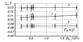
Fig. 3. Dependence of the adhesion component of the friction factor  $f_a$  (curves 1, 2) and the friction factor f after the micro running-in (curve 3) on contour pressure  $p_C$  for surfaces without micro grooves
