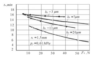
Fig. 13. Dependence of the time of the micro running-in completion  $t_w$  on the relative area of micro grooves  $F_k$
