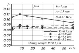
Fig. 9. Dependence of the adhesion component of the friction factor  $f_a$  on the roughness  $R_Z$  of the sample carrying surface
