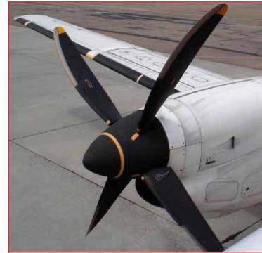
Fig. 6. Propeller in a feathered position
