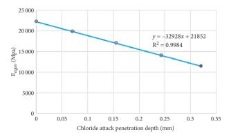
Figure 7. Variation of Eequv and chloride attack penetration depth
