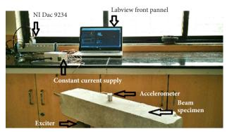
Figure 4. Laboratory setup to measure first natural frequency
