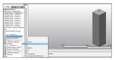
Figure 5. 3D beam specimen with meshing
