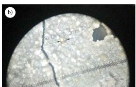
Figure 3. Beam crack measurement: a – Crack width measuring pocket microscope; b – Crack width under microscope
