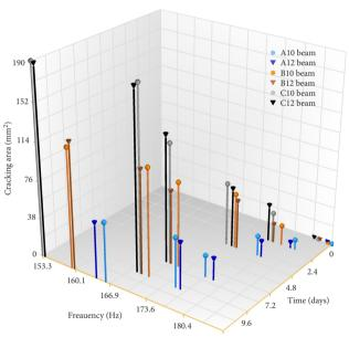
Figure 10. 3D graph for first natural frequency, cracking area, test time of accelerated corrosion
