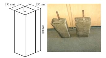
Figure 1. Beam specimen with dimension: a – Symmetrical representation of beam specimen; b – Casted beam specimens as per the symmetry
