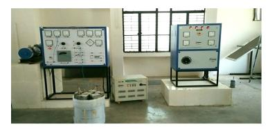
Figure 2. Laboratory setup of accelerated method of corrosion using impressed current technique
