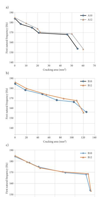
Figure 9. Natural frequency (Hz) versus cracking area (mm²): a – First natural frequency vs cracking area of beam A10, A12; b – First natural frequency vs cracking area of beam B10, B12;
