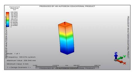
Figure 6. First natural frequency of beam A10
