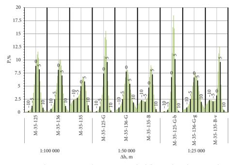
Fig. 5. SRTM Elevation Error Distribution Histogram for different scales and terrain conditions
