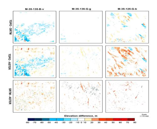
Fig. 4. The rasters of surface's difference according to different sources of DTM data
