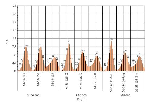
Fig. 6. ASTER GDEM Elevation Error Distribution Histogram for different scales and terrain conditions
