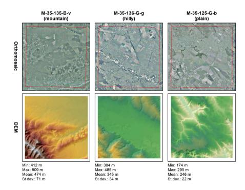
Fig. 2. Elevation characteristics of the researched polygons
