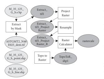
Fig. 3. ArcGIS geoprocessing model for the elevation difference raster generation
