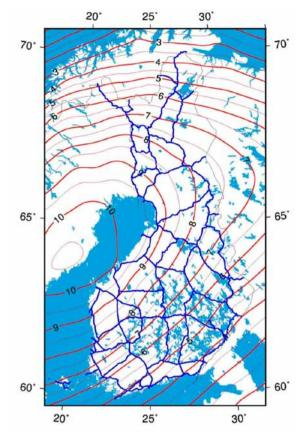
Fig. 1. Postglacial rebound in Finland (red contours), in mm/year. The contours are from the Nordic uplift model NKG2005LU (Vestøl 2005; Ågren, Svensson 2007), which is relative to the Baltic mean sea level 1892–1991. The model is adjusted in vertical direction to fit the GNSS based absolute uplift rate by Lidberg *et al.* (2007). The first order levelling network (N2000) is in blue lines
