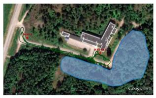
Fig. 2. Aerial photograph of the test field presenting the location of the benchmarks, harvested trees (blue polygon) and the trajectory from the MLS measurements (green dotted curve) (image: Google Earth)
