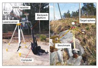
Fig. 6. The MLS system Akhka R2 (left) and a white sphere adjusted above the benchmark 95011 (right)
