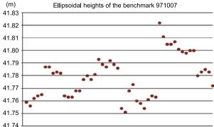
Fig. 4. Variations of the VRS height measurements on the benchmarks
