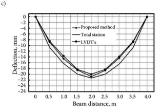
Fig. 3. Plots of the beam deflections for a) 0.5 ton load, b) 1.0 ton load and c) 1.5 ton load
