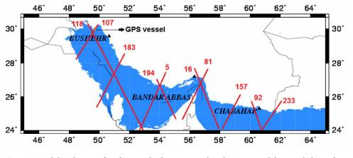
Fig. 2. Spatial distribution of study coastal tide gauges, within the Iranian tidal network, located at Bushehr, Bandar Abbas and Chabahar ports, GPS vessel deployment, and the altimetry ground tracks
