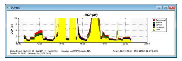
Fig. 4. Value of DOP criteria for the point 001 with the horizon closedness 42% received from the program planning
