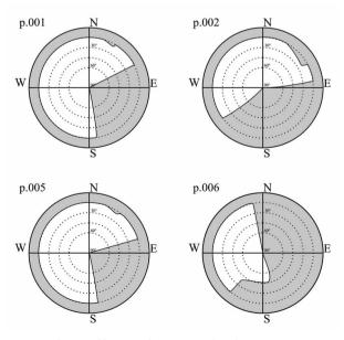
Fig. 3. Scheme of barriers location at the observations points (Yanchuk 2014)
