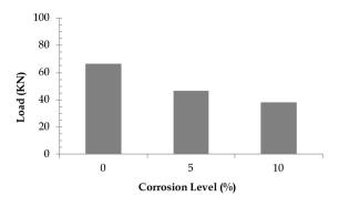
Fig. 8. Effect of corrosion level on load carrying capacity of series A beams
