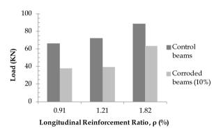
Fig. 9. Effect of corrosion on load carrying capacity of beams with different reinforcement ratios
