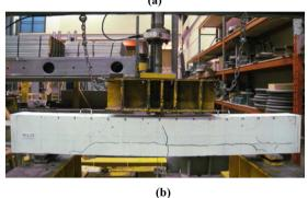
Fig. 7. Failure modes: a) Control beam (N-1.21); and b) Control beam (M-1.21)
