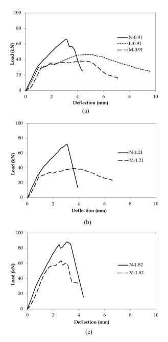
Fig. 6. Load deflection behaviour of tested beams: a) series-A; b) series-B; c) series C
