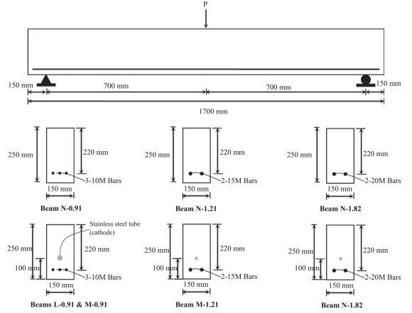
Fig. 1. Details of test specimens and loading arrangement
