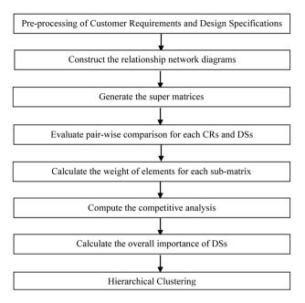
Fig. 2. Flow chart of the proposed fuzzy ANP-QFD method with hierarchical clustering
