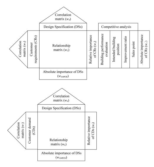
Fig. 1. QFD framework of the hybrid QFD- FANP method
