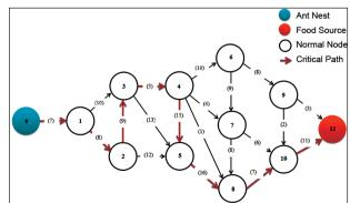
Fig. 3. Network Diagram for Final Solution of CPM
