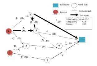
Fig. 4. Network topology result in Step 1 using CSAM-ACO acceleration model
