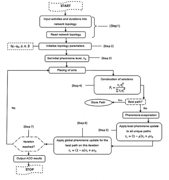
Fig. 1. ACO algorithm processes for the development of CSAM-ACO acceleration model
