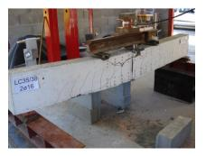
Fig. 3. Test beam after failure
