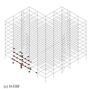
Fig. 5. Member failure and plastic hinge locations for horizontally irregular MRF, CBF, EBF – Blast Location 1
