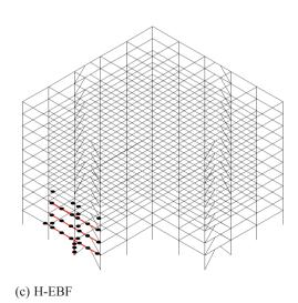
Fig. 6. Member failure and plastic hinge locations for horizontally irregular MRF, CBF, EBF – Blast Location 2
