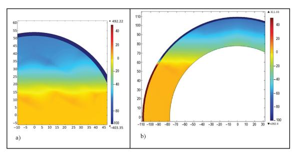
Fig. 3. a) Position of the plastic neutral axis in circular composite beams with a solid concrete core ( $\emptyset$ 108×2.25); b) in circular composite beams with a hollow concrete core ( $\emptyset$ 219×1.6)
