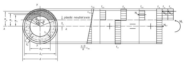
Fig. 1. Diagrams of linear strain and ideally plastic stress distributions in the hollow concrete-filled steel tubular cross-section
