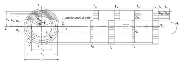
Fig. 2. Stress distribution in the steel and concrete circular cross-sections experiencing bending, taking into account tension of the concrete core
