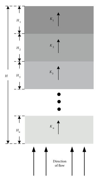
Fig. 2. The configuration of water flow through layered soils in the FDM formulation
