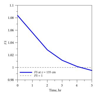
Fig. 14. The computed results of FS at z = 135 cm for application example 2
