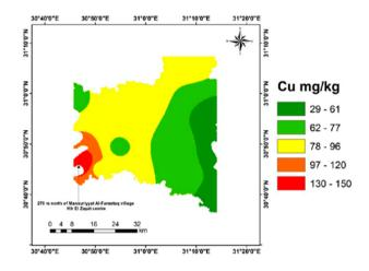
Fig. 7. Spatial interpolation of the weighted mean of copper
