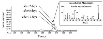
Fig. 2. Chromatogram of chlorothalonil degradation in apples after 2, 5 and 15 days for the phenological stage 30–40 mm fruit size (BBCH 74)
