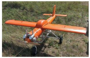
Fig. 2. The "MOA-1" unmanned aerial vehicle
