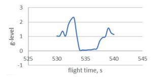
Fig. 4. Typical g- level test result during simulator parabola fight
