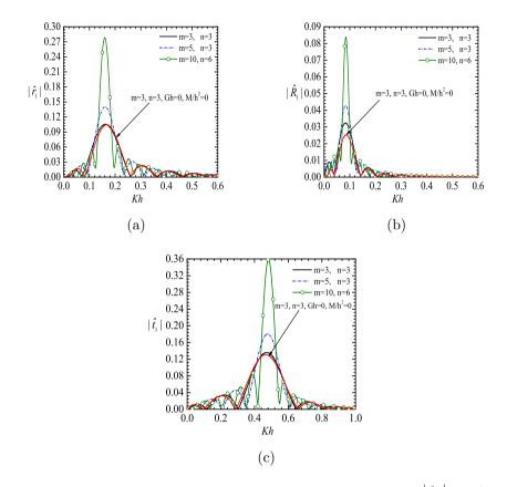
Figure 5. Coefficients due to incident wave of mode  $\lambda_2$  in (a)  $|\hat{r}_1|$ ; (b)  $|\hat{R}_1|$ ; (c)  $|\hat{t}_1|$  for H/h = 2, a/h = 0.1,  $\gamma h = 1$ ,  $\rho = 0.5$ ,  $M/h^2 = 0.2$ , Gh = 0.05.
