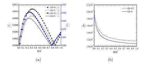
Figure 7. Coefficients due to incident wave of mode  $\lambda_2$  in (a)  $|\hat{r}_1|$  and  $|\hat{t}_1|$ ; (b)  $|\hat{R}_1|$  for  $\rho = 0.5, H/h = 2, Kh = 0.5, \gamma h = 1, a/h = 0.1, m = 5, n = 3.$
