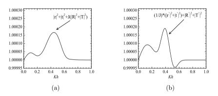
Figure 12. (a)  $|r|^2 + |t|^2 + J(|R|^2 + |T|^2)$  versus Kh, and (b)  $\frac{1}{J}(|\hat{r}|^2 + |\hat{t}|^2) + |\hat{R}|^2 + |\hat{T}|^2$  versus Kh for  $\rho = 0.5$ , H/h = 2,  $M/h^2 = 0.2$ .
