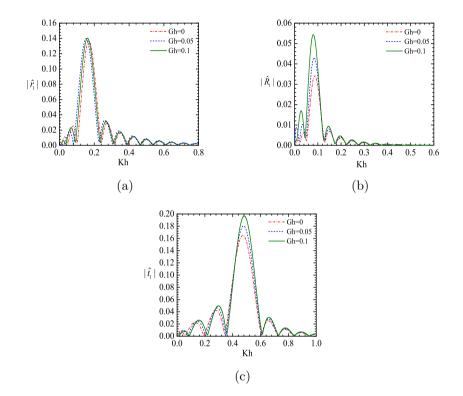
Figure 9. Coefficients due to incident wave of mode  $\lambda_2$  in (a)  $|\hat{r}_1|$ ; (b)  $|\hat{R}_1|$ ; (c)  $|\hat{t}_1|$  for  $\rho = 0.5, H/h = 2, M/h^2 = 0.2, \gamma h = 1, a/h = 0.1, m = 5, n = 3.$
