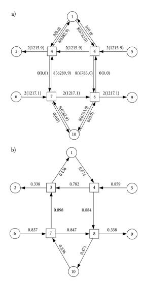
Fig. 5. The solutions for network capacity problem with Strategy 2: a – optimal link flow solution (in brackets) and number of lanes (out of brackets) for network capacity problem with Strategy 2; b – the Volume/Capacity (V/C) at maximum network capacity state of Strategy 2
