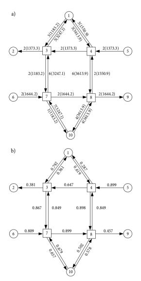
Fig. 4. The solutions for network capacity problem with Strategy 1: a – optimal link flow solutions (in brackets) and number of lanes (out of brackets) for network capacity problem with strategy 1; b – the Volume/Capacity (V/C) of each link at maximum network capacity state of Strategy 1
