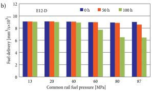
Fig. 3. High pressure pump fuel delivery versus common rail fuel pressure
