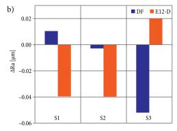
Fig. 4. Plungers surfaces  $\Delta R_a$  and  $\Delta R_z$  values for both tested fuels
