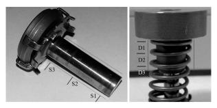
Fig. 2. Location of the points used for surface roughness and surface microstructure analysis
