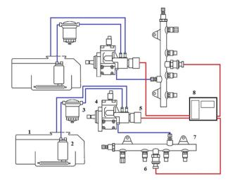
Fig. 1. Experimental test bed scheme: 1 – fuel tank; 2 – fuel transfer pump; 3 – fuel filter; 4 – high pressure pump; 5 – fuel (rail) pressure regulator; 6 – fuel pressure sensor; 7 –common rail; 8 – fuel pressure control unit
