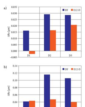
Fig. 5. Barrels surfaces  $\Delta R_a$  and  $\Delta R_z$  values for both tested fuels
