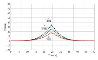
Fig. 3. Simulation result of contact wire uplift waveform for three trains of speed  $\nu = 3.6$  m/s, each with one raised pantograph with different adjusted static forces
