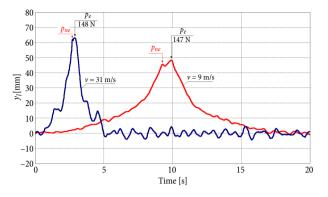
Fig. 14. Contact wire uplift waveform for the same locomotive with two raised pantographs inter-spaced extremely closely at  $l_{1-2} = 5$  m, tested in consecutive days with varying train speeds detected
