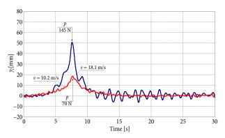
Fig. 12. Comparison of measurement results of contact wire uplift waveform for two trains, each with one raised pantograph p: the first train of excessive static force of current collector and an insufficient value for the second
