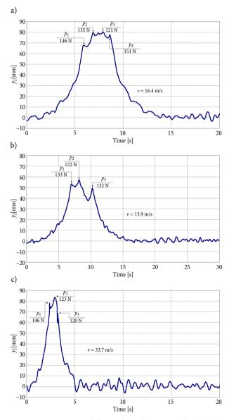
Fig. 13. Contact wire uplift waveform for trains with multiple raised pantographs p based on the following inter-spacing
