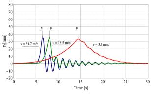
Fig. 4. Simulation result of contact wire uplift waveform for three trains, each with one raised pantograph of static force  $F_u = 130$  N, distinguished by different train speeds
