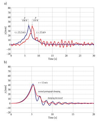
Fig. 15. Contact wire uplift waveform for trains with one raised pantograph *p*: a – measurement results in cases of minimally and greatly excited oscillations of the wire;
