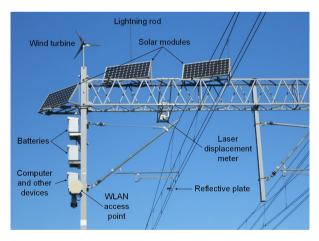
Fig. 7. Measuring station on catenary support structure
