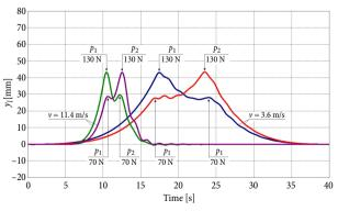
Fig. 6. Simulation results of contact wire uplift waveform for four trains, each with two raised pantographs  $p_1$ ,  $p_2$  spaced at  $l_{1-2} = 24$  m of strongly differing static forces:  $F_{u1-A} = F_{u2-B} = F_{u1-C} = F_{u2-D} = 130$  N and  $F_{u2-A} = F_{u1-B} = F_{u2-C} = F_{u1-D} = 70$  N
