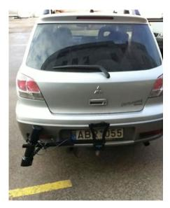
Fig. 4. Sensor for measurement of friction (RCM 411) installed on a tow-ball of a vehicle (Bulevičius *et al.* 2014)
