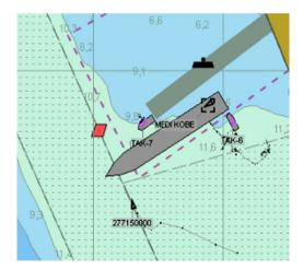
Fig. 8. A mooring ship partly blocks current flow and decreases the cross square of the channel
