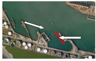
Fig. 3. Jetties for the oil terminal at the Port of Le-Havre and directions of tidal currents
