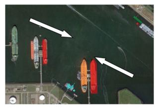
Fig. 2. Jetties for the oil terminal at the Port of Rotterdam and directions of tidal currents
