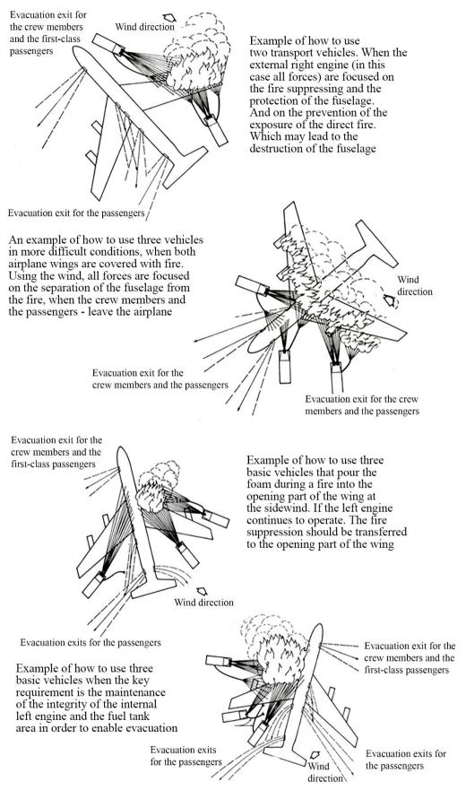
Figure 1. Possible situations related to airplane in case of accidents with fire and evacuation scenarios (ICAO-Montreal, 2011)
