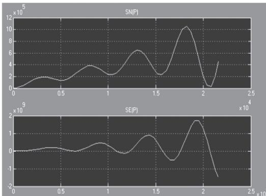
**Fig. 11.** Graphs of errors on both channels traversed the path of inertial systems when there is cross-connection between the channels due to transfer coefficients  $kn_{pv} = 0.001$ ,  $kn_{pv1F} = 0.001$ ,  $kn_{pv2F} = 0.001$ , and  $kn_{pv} V_2 = 0.0001$
