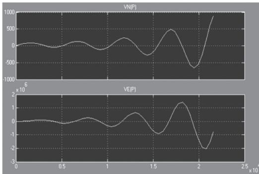
**Fig. 10.** Graphs of error rates of the two channels of an inertial system when between the channels there are cross-connections with coefficients of transmission  $kn_{pv} = 0.001$ ,  $kn_{pv1F} = 0.001$ ,  $kn_{pv2F} = 0.001$ , and  $kn_{pv} V_2 = 0.0001$
