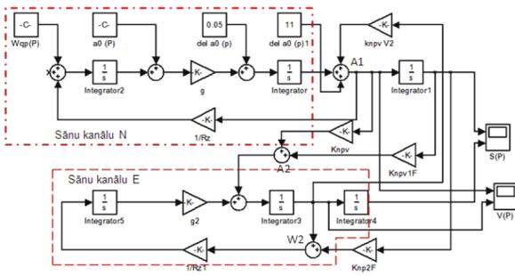
Fig. 6. Model of inertial system errors when two channels jointly operate
