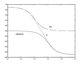
Fig 7. Bode diagrams for systems pilot-airplane in the heading channel for classical plane and for heading oriented control if PD-type or P-type heading rate regulator used
