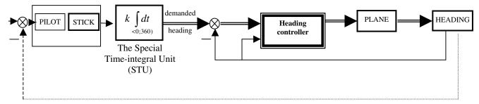
Fig 8. The schematic of the Heading Rate Control Heading Keep (HRCHK) algorithm
