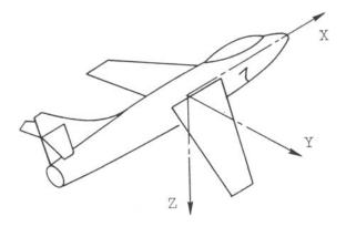
Fig 2. The airplane axis system with its origin located in plane's center of gravity
