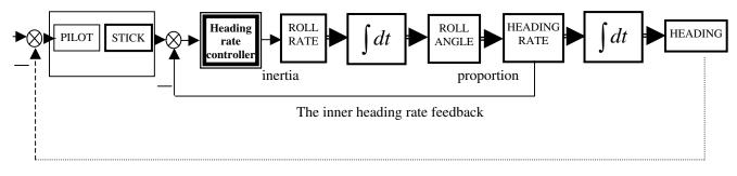
Fig 6. The schematic of the pilot-airplane system in the heading-oriented case of the control
