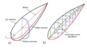
Fig. 3. Concept of fuselage definition
