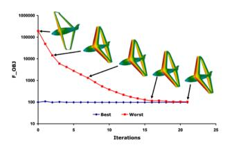
Fig. 10. Optimization of joinwing aircraft geometry.
