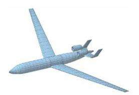
Fig. 8. Grid of innovative transport aircraft.
