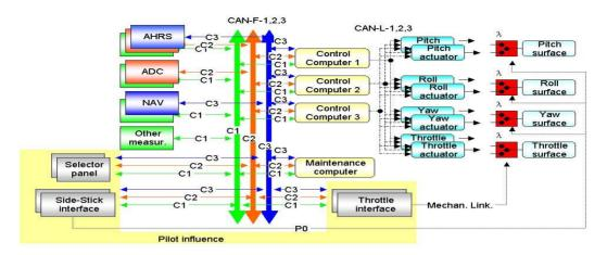
Fig 2. General structure of the fly-by-wire flight control system for PZL-104
