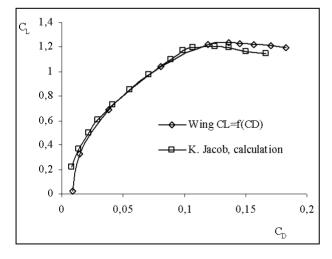
Fig 10. Lift-drag characteristics for a NACA 4415 rectangular wing with AR=6.2 at Re=2.1x106. Experimental results were used as 2D section data
