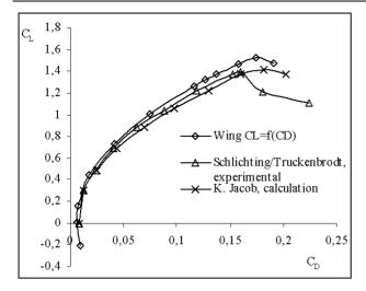
**Fig 9.** Lift-drag characteristics for a NACA 2412 rectangular wing with AR=5 at Re=2.7x106. X-FOIL calculation results were used as 2D section data
