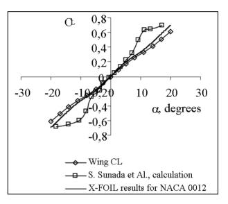
Fig 8. Lift coefficient of NACA 0012 rectangular wing with AR=7.25 at Re=4000. X-FOIL calculation results were used as 2D section data
