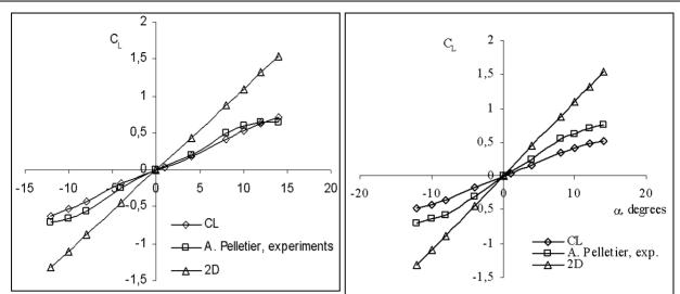
Fig 1. Lift coefficient of a flat plate rectangular wing of aspect ratio 3, at Re=80000. For calculation, section experimental results were used
