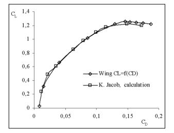
Fig 11. Lift-drag characteristics for a NACA 4415 not tapered swept wing (20 deg.) with AR=6.2 at Re=2.1x106. Experimental airfoil results were used as 2D section data
