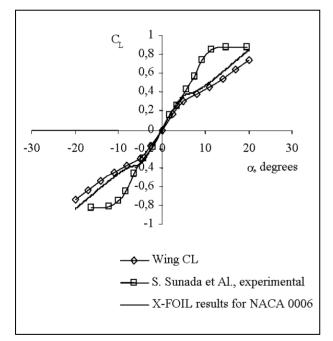
Fig 6. Lift coefficient of NACA 0006 rectangular wing with AR=7.25 at Re=4000. X-FOIL calculation results were used as 2D section data
