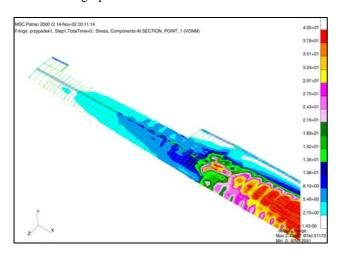
Fig 10. Effective stress concentration (von Misses) around wingtip and centre wing connection
