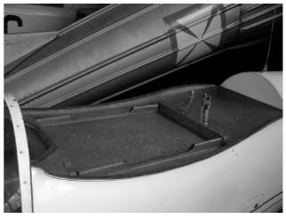
Fig 16. Clasps for attaching pins in fuselage centre section
