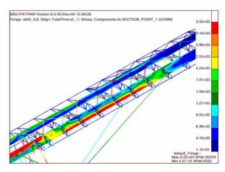
**Fig 6.** Effective stress in main spar (von Misses). Tension of bottom strips at level of 350[MPa]
