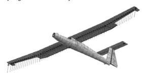
**Fig 9.** Forces and constrains simulating symmetrical steady flight
