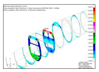
Fig 15. Effective stress distribution (von Misses) in fuselage carrying frames in fuselage – wing joints
