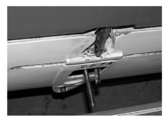
**Fig 14.** Relief for the beam and vertical pilot bar mounted into the stabilizer spar
