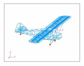
Fig 3. The numerical model of light airplane structure
