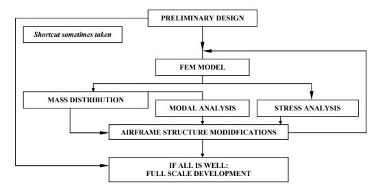
Fig 1. Algorithm of numerically supported preliminary design
