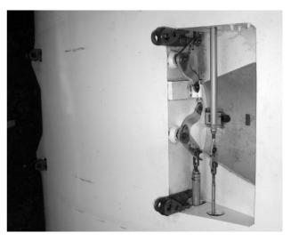
Fig 17. Four-point joints in centre wing
