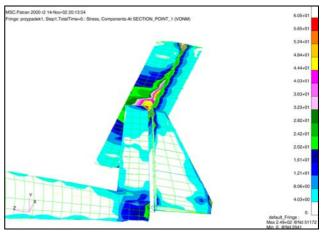
Fig 12. Effective stress concentrations (von Misses) in empennage connection
