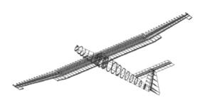
Fig 8. The sailplane geometry (covering is not shown)
