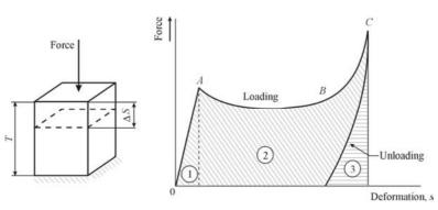
Fig 2. Force and shift interdependence of porous composite
