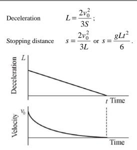
Fig 8. Rate of deceleration with a triangular form (No 1)
