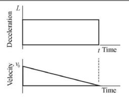
Fig 10. Rate of deceleration with a triangular form (No 3)
