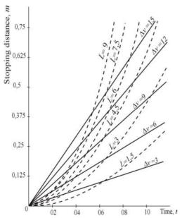
Fig 3. Stopping distance and time interdependence of speed change and deceleration level
