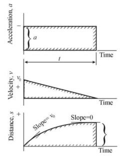
**Fig 4.** Rate of deceleration with a rectangular form Here
