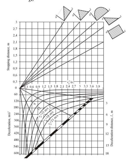
Fig 12. The dependences of the velocity, the deceleration and the distance on the time
