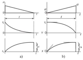
**Fig 5.** A deceleration rate of triangular form a – sag till zero time; b – level till zero time
