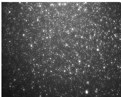
Figure 4. Fluorescence microscopy (zoom \times 200 ) images of bitumen after ageing (RTFOT + PAV)
