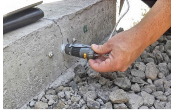
Figure 3. Measurements of LTE and crack width in test section of short concrete slabs
