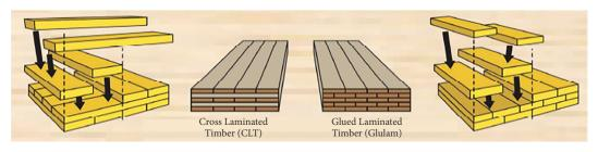
Figure 1. Difference between CLT and glulam (Avellan, 2018)
