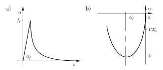
Figure 5. Graphs of masonry units' material parameters in numerical model: a) exponential function; b) parabolic function (according to TNO Diana, 2011)
