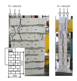
Figure 1. Failure mode of compressed masonry under bearing load 684 kN
