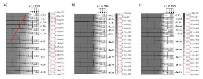
Figure 7. Distribution of main compressive stresses: a) at load of 1 MPa; b) at load of 10 MPa; c) at load of 15 MPa
