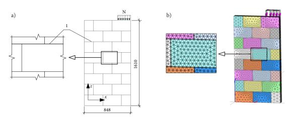
Figure 4. Numerical model of calcium silicate blocks masonry fragment: a) dimensions of fragment; b) numerical model of wall with finite elements net: 1 – blocks contact area
