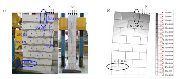
Figure 8. Cracks distribution and crack formation loads: a) experimental research; b) numerical modeling
