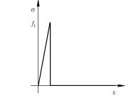
Figure 6. Failure mode of mortar joint in numerical model
