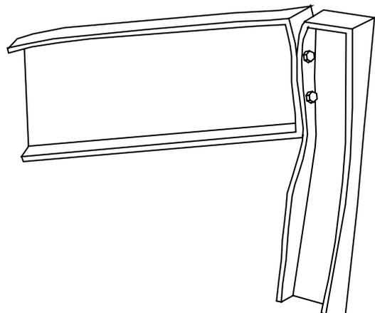
Fig. 4. An example of a real semi-rigid joint
