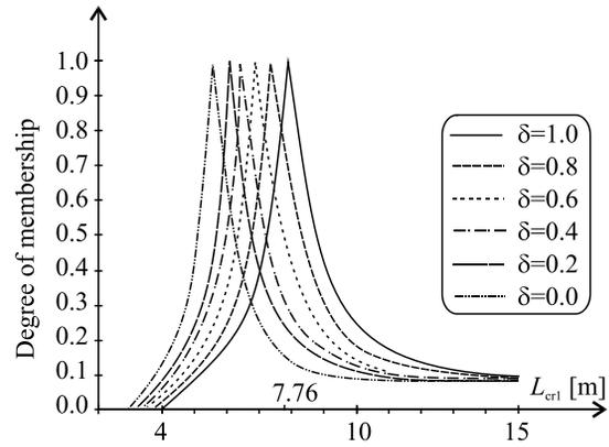
Fig. 8. Fuzzy buckling length of the left column
