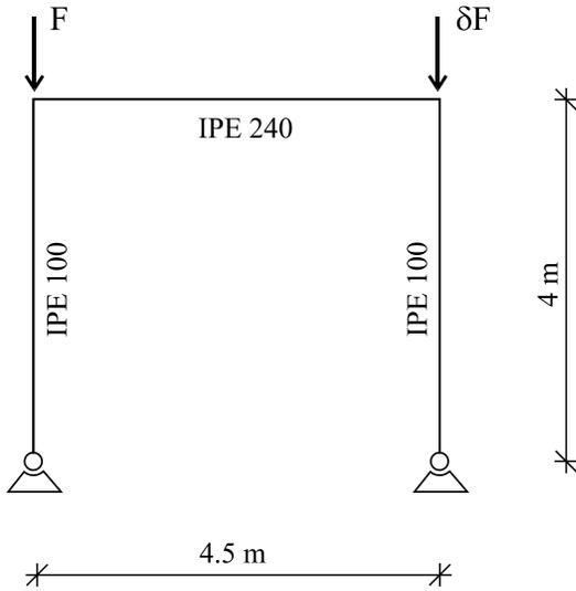
Fig. 1. The geometry of a steel plane frame
