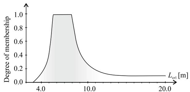
Fig. 10. Fuzzy buckling length of the left column
