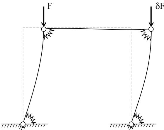
Fig. 2. Buckling a frame with a semi-rigid joint
