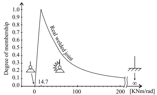
Fig. 3. Stiffness of support joints
