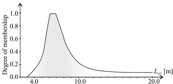
Fig. 13. Fuzzy buckling length of the left column
