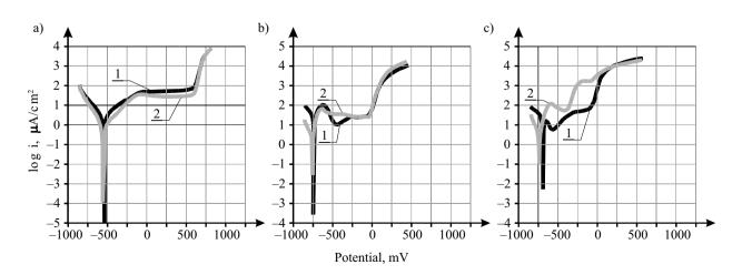
**Fig. 4.** Polarization curves of reinforcing steel in model solution: 1 – without inhibitor, 2 – with M preparation. Description in the text
