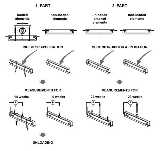
Fig. 11. Course of second stage tests with advanced reinforcement corrosion
