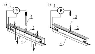
**Fig. 6.** Scheme of polarization measurements in the beams: a) loaded and cracked, b) unloaded. Description in the text
