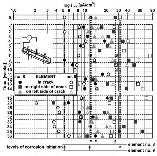
Fig. 13. Results of electrochemical tests on reinforcement with advanced corrosion in loaded and cracked comparative elements without inhibitor: a) number 8, b) number 97
