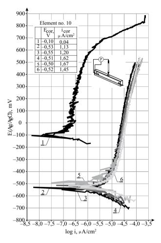
Fig. 15. Polarization curves obtained in unloaded element number 10 protected with KCR inhibitor: 1 – in passive state before corrosion initiation, 2 – after initiation of corrosion, 3 – directly after inhibitor application, 4 – after 9 weeks of inhibitor action, 5 – after second inhibitor application, 6 – at the end of the measurements
