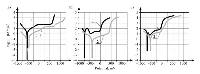
**Fig. 3.** Polarization curves of reinforcing steel in model solution: 1 – without inhibitor, 2 – with KCR inhibitor. Description in the text
