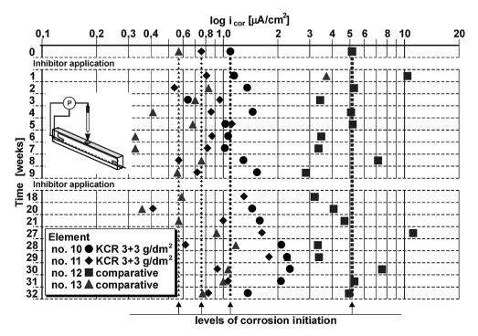
Fig. 14. Results of electrochemical tests on reinforcement with average corrosion in unloaded element numbers 10 and 11 saturated with KCR inhibitor and numbers 12 and 13 without inhibitor
