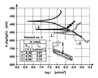
Fig. 10. Polarization curves obtained from element number 2:
