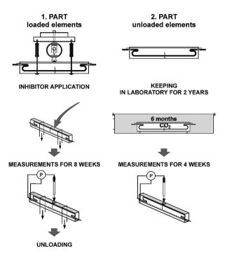
Fig. 8. Course of first-stage tests with marginal reinforcement corrosion
