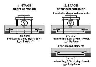
Fig. 7. Method of reinforcement corrosion initiation
