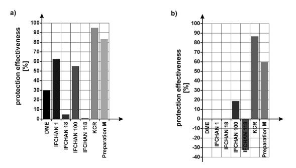
**Fig. 2.** Effectiveness of inhibitors in carbonated and chloride contaminated solution: a) mixture of NaOH, KOH and  $Ca(OH)_2$  hydroxides, b) extract of hardened cement past
