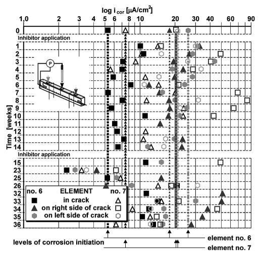
**Fig. 12.** Results of electrochemical tests on reinforcement with advanced corrosion in KCR saturated inhibitor, with loaded and cracked elements: a) number 6, b) number 7
