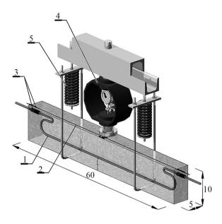
Fig. 5. Scheme of element structure and way of loading
