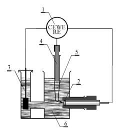
Fig. 1. Scheme of the measuring system: 1 – potentiostat,
