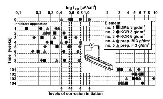
**Fig. 9.** Results of tests on inhibitor effectiveness in elements with a low level of development in reinforcement corrosion processes
