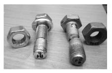
Figure 3. Facture modes of the non-preloaded regular bolts (on the left) and high strength bolts (on the right)
