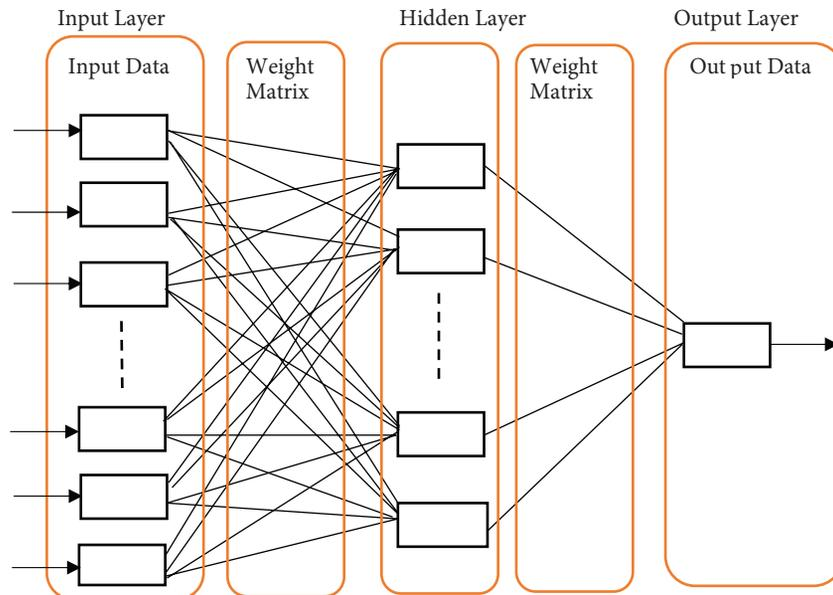
Figure 3. Basic BPNN structure
