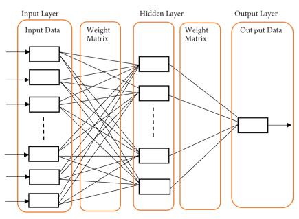
Figure 3. Basic BPNN structure
