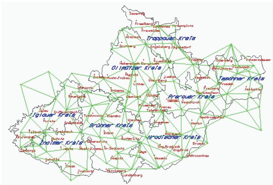
Fig. 3. Trigonometric Net of I<sup>st</sup> order
