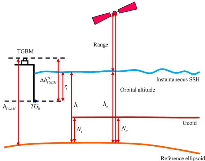
Fig. 1. Schematic view of relations between instantaneous sea surface heights measured by coastal tide gauge from the tide gauge reference point ( $TG_0$ ) with respect to the reference ellipsoid and geoid
