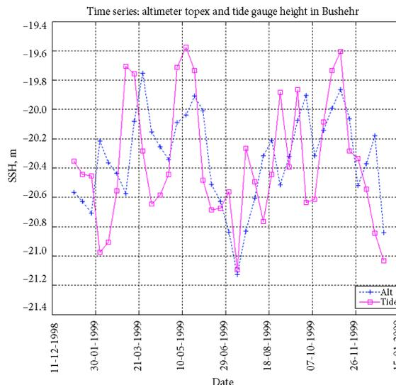
Fig. 5. SSH time series obtained from Topex/Poseidon against those of Bushehr tide gauge over a 1-year time span from 1999 to 2000
