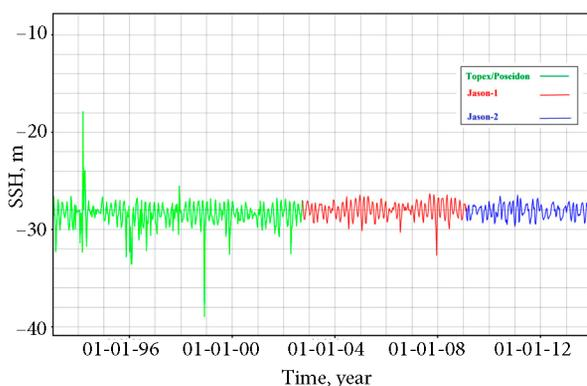
Fig. 4. Altimetry SSH time series at Bandar Abbas port derived from Topex/Poseidon, Jason-1 and Jason-2 over a 22-year span from 1993 to 2014
