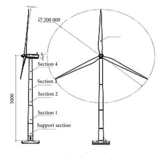
Figure 3. Scheme of a wind turbine
