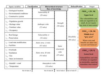
Figure 3. Hierarchical structure of Fuzzy Building Service Life extended (*FBSL*<sub>2,0</sub>) (Prieto et al., 2019)
