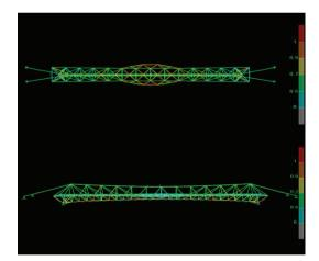
Figure 27. The graphical representation of the loads in the structural members
