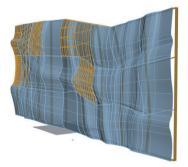
Figure 2. Entire wall panel sized 540x210 cm where several cells have applied the early stage cuts in non-standard angles
