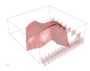
Figure 1. Construction planes are set on x-axis and y-axis to cut any complexity of surfaces into regular contours
