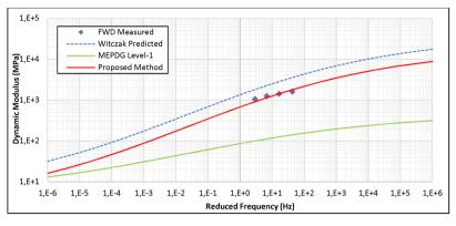
Fig. 5. Dynamic modulus master curves of asphalt layer for Site S01
