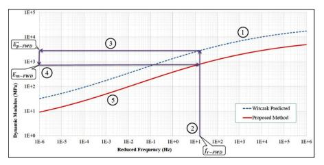
Fig. 1. Procedure of proposed method for development of in-situ |E\*| master curve
