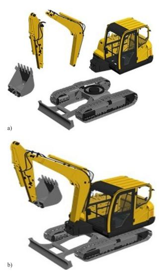
Fig. 2. a) 3D models of the excavator sections; b) equipment configuration
